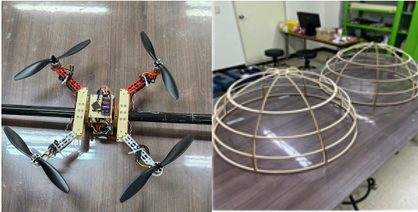
Fig. 2. Quadrotor without shell(Left), Hemisphere shell(Right)
