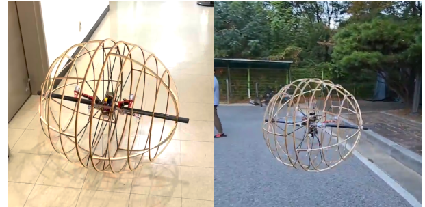
Fig. 4. Free moving on the ground(Left), Hovering (Right)
